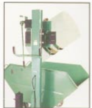
Manual crank offers quick, easy 360° rotating and controlled dumping to either side.
