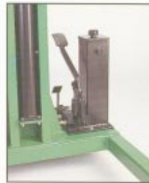
Manually powered models to utilize a foot-powered hydraulic pump for lifting. Lifting speed 5 fpm.
