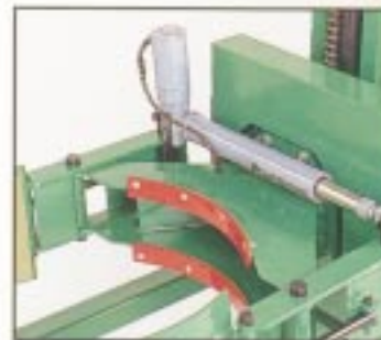
Electric operated screw-jack is used to clamp and release the rubber lined jaws.
