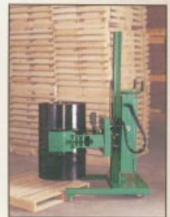
The Roto-Grip can also pick drums off of the corner of a pallet.
